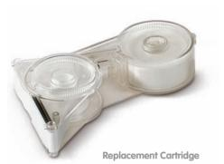
The CleanCore cassette is supplied with a removable cartridge containing the cleaning fabric. The cartridge supports 400 cleaning cycles. Replacement cartridges can be purchased and installed into the CleanCore cassette, by simple unscrewing two retaining screws on the side of the unit. The cleaning fabric has a super fine cross woven weave, which permits dry cleaning of a fibre optic connector end face, through the simple action of two wipes down the length of exposed cleaning fabric.
