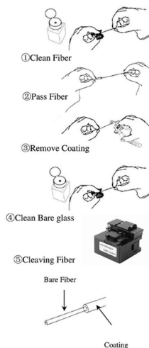
Fig. 3-3 Fiber Stripping
